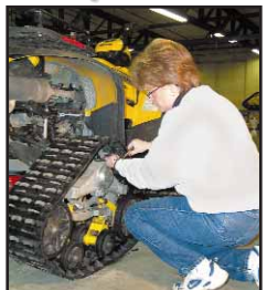
2. Position track and attach the wheel bolts and the rubber anti-torque linkage.
